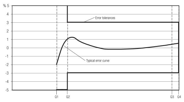
$Q_1 < Q < Q_2$  lower measuring range Q2 < Q< Q4 upper measuring range
